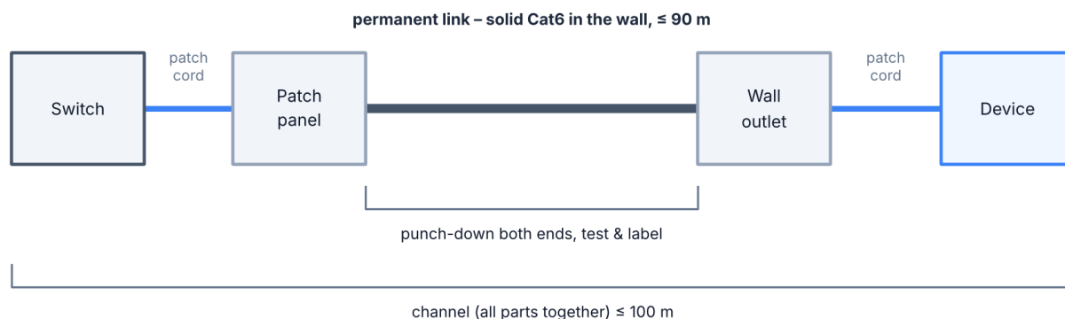
Figure 6.1 Structured cabling: a fixed permanent link in the wall, short patch cords at both ends.
